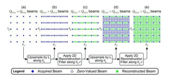
*Application Of Separable 2-D Filters For 3-D Image Reconstruction. Each Point Represents A Single Beam That Extends Radially From The Center Of The Array.*
