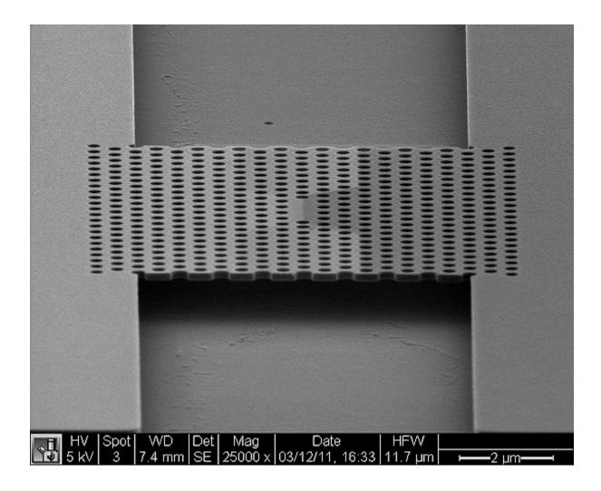
SEM of photonic crystal nanocavity Image courtesy of Jelena Vuckovic
