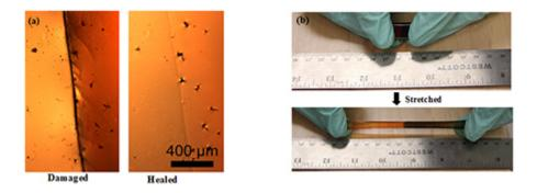
**Self-healing properties of the polymer film.** Photographs of (a) damaged and healed samples and (b) healed film before and after stretching.
