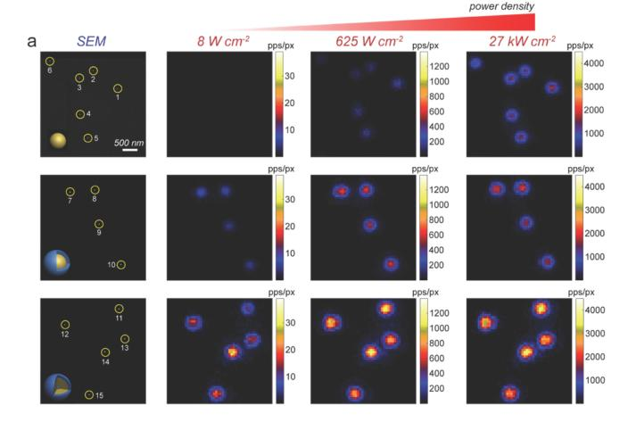
**Figure 1**. (a) Correlation between SEM and power density-dependent wide-field fluorescence images for three types of UCNP: (top row) 22.0 nm  $\text{NaY}_{0.78}\text{F}_4:\text{Yb}_{0.2}\text{Er}_{0.02}$ , (middle row) 29.1 nm  $\text{NaY}_{0.78}\text{F}_4:\text{Yb}_{0.2}\text{Er}_{0.02}$ @  $\text{NaYF}_4$ , (bottom row) 29.4 nm  $\text{NaYF}_4$ @NaYb\_{0.92}F\_4:Er\_{0.08}@NaYF\_4.
