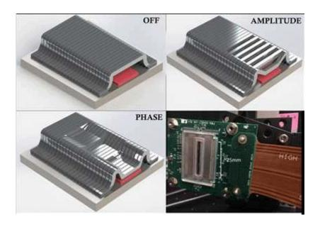
**Phased Array for Random Access Scanning:** Model of phased array with silicon ribbons in passive state (off) and active operation (amplitude and phase). By controlling the ribbon with small voltages, the device acts as a diffraction grating for pulsed laser light.
