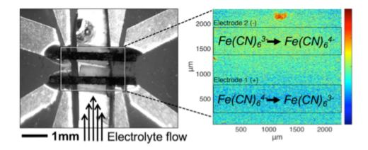
Redox refrigerator device electrodes and electrolyte flow channel in optical and IR views.
