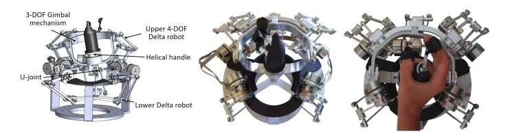
Compact and High-Fidelity Device for Versatile Haptic Teleoperation The mechanical transparency of the design and its novel paired parallel structure meet the challenge of accuracy, stiffness, and haptic capability required in remote tasks.
