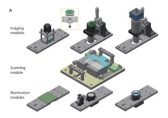
**Figure description -** Low-cost, open source and modular automated scanning/tracking fluorescent microscope. (A) Construction of the modular microscope with swappable parts.
