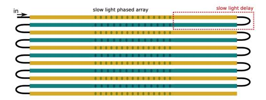
Figure 1 Matched slow light waveguide serpentine OPA architecture (Image courtesy the Vuckovic Group)
