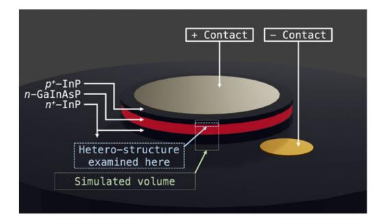
Image description: A depiction of the fabricated device highlighting the heterojunction used to enhance performance. Ref: Santhanam et al. Applied Physics Letters (2020)
