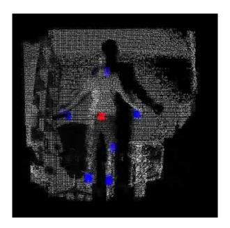
This <u>video</u> shows test data of body part detection via active motion capture. Experiments showed that this system is significantly better at detecting body parts in depth images than state-of-the-art sliding-window based detectors.
