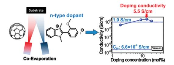
Conductivity of n-Type Dopant 2-(2-Methoxyphenyl)-1,3-dimethyl-1H-benzoimidazol-3-ium Iodide Image Courtesy the Bao Group
