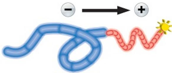
*This schematic of FSCE shows the monodisperse protein drag-tag (blue) conjugated to the DNA sequencing fragment (red) with fluorescent dye attached for detection (yellow star). Covalent attachment of the drag-tag to the DNA molecule allows for size-based separation in an electric field with no sieving matrix.*
