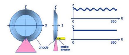
**Figure description -** The optimal number of "hills" and "valleys" on the anode depends on the anode rotation speed and the DAS speed.
