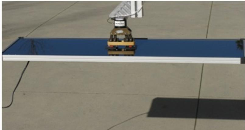
A custom end-effector using the adhesives being used to support a large solar panel.
