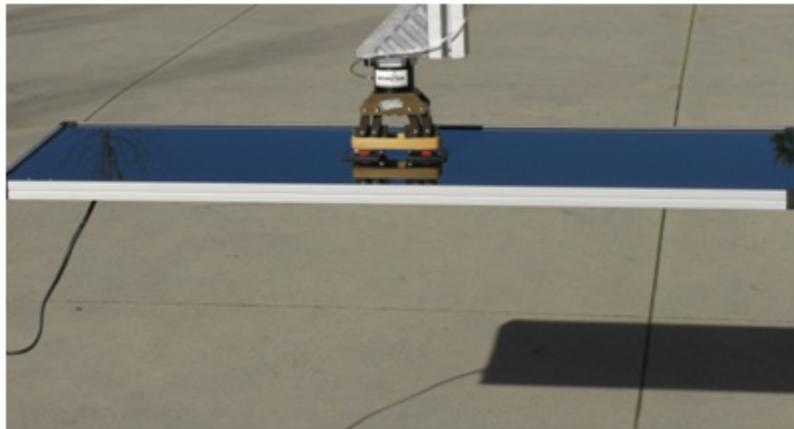
A custom end-effector using the adhesives being used to support a large solar panel.
