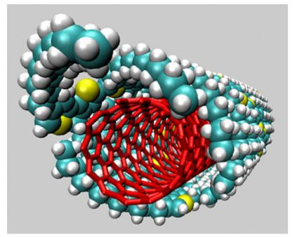
Schematic of the polymer (blue) wrapped around the semiconducting single walled carbon nanotube (red)
