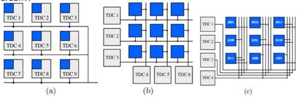
Three SiPM designs with: (a) one TDC (time to digital converter) per pixel, (b) one TDC per row and column of pixels, and (c) one TDC per bit of the binary representation of each pixel number.
