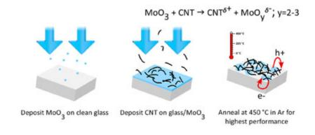
**Figure description -** Schematic showing the fabrication of MoOx-CNT transparent conductors.
