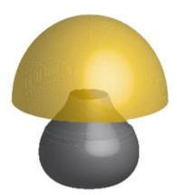
**Schematic of thermal extraction.** Thermal extraction using a hemispherical refracting dome placed at the opening of a high-index thermal cavity, which in practice may be simply the surface of an emitting solid. The dome is transparent and does not emit or absorb any thermal radiation. Many other geometries are also
