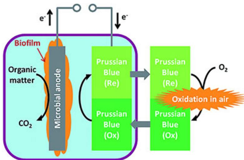
**Schematic of the microbial battery (MB) equipped with a Prussian Blue (PB) cathode.** *The microbial anode produces electrons from organic matter. The electrons flow to the PB electrode that functions as a cathode and is reduced. When exposed to oxygen in air, the reduced PB is re-oxidized.*
