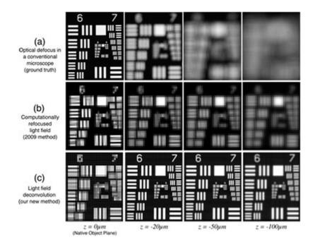
Comparison of conventional (a) and LFM (b and c) imaging of USAF 1951 resolution test target translated to depths up to 100 um from the native object plane (z = 0 um). The wave optics reconstruction algorithm (c) improves lateral resolution up to 8-fold compared to standard LFM imaging (b), except at the z = 0 plane (left image).
