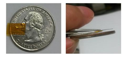
Figure description - World's smallest pressure sensor at 1×1×0.1 mm
