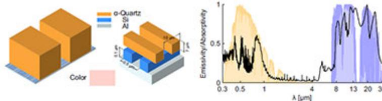
*On the left is a schematic drawing of radiative cooling structure which includes a quartz bar array on top of silicon nanowires. On the right, the black curve shows the emissivity/absorptivity spectrum of the modified structure.*
