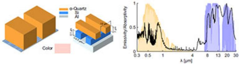
*On the left is a schematic drawing of radiative cooling structure which includes a quartz bar array on top of silicon nanowires. On the right, the black curve shows the emissivity/absorptivity spectrum of the modified structure.*
