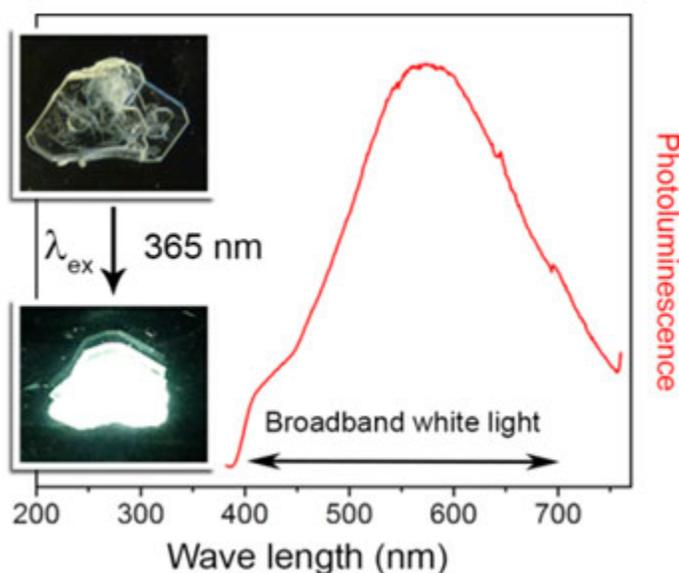
**Figure description** - Broadband white-light photoluminescence (PL) from a single crystal of (EDBE)[PbBr<sub>4</sub>] under near-UV irradiation.
