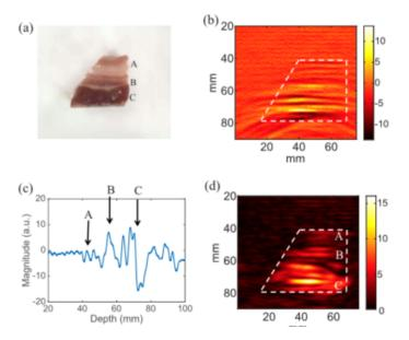
**Figure Description** (a) Pork belly tissue used in the experiment. (b) 2D raw matched filtering image. (c) 1-D matched-filtering result between measured signal and transmit reference signal. (d) Reconstructed image using FD-SAR. In the figures, A-C denote the top skin, middle muscle, and bottom muscle layers.
