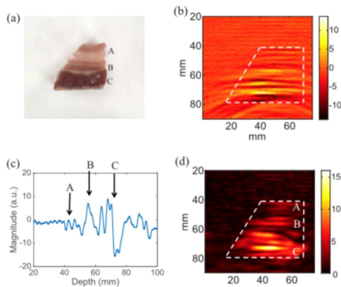
**Figure Description** (a) Pork belly tissue used in the experiment. (b) 2D raw matched filtering image. (c) 1-D matched-filtering result between measured signal and transmit reference signal. (d) Reconstructed image using FD-SAR. In the figures, A-C denote the top skin, middle muscle, and bottom muscle layers.
