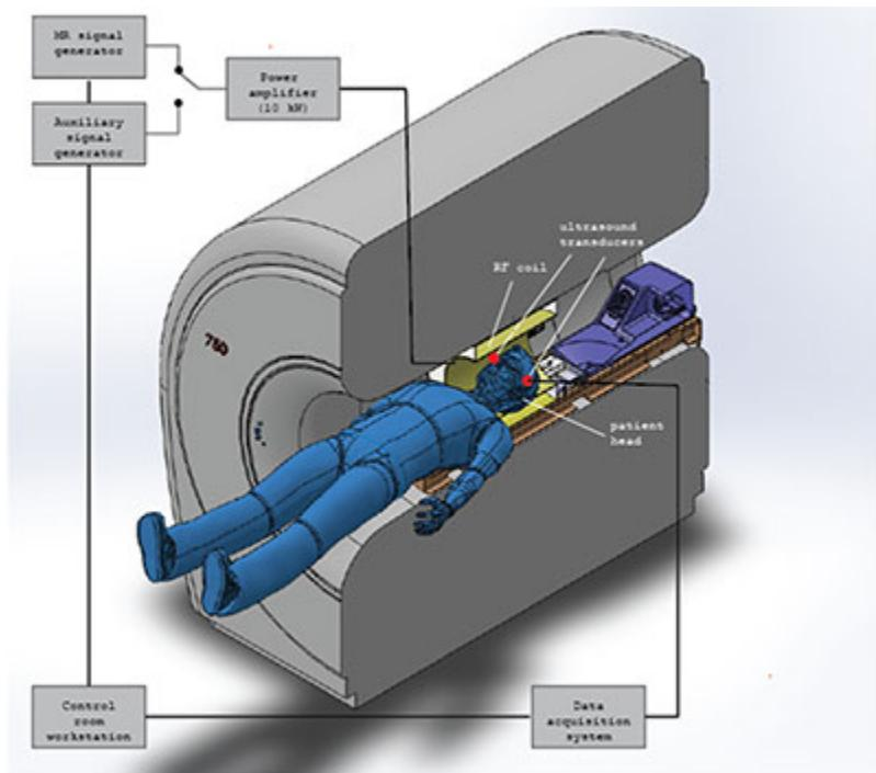
**Fig. description:** MR scanner with proposed closely coupling ultrasound transducer configuration.
