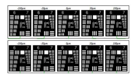
Comparison of LFM imaging of USAF 1951 target. Top- no phase mask. Bottom-with phase mask. The resolution at the native object plane (0um) is improved with the phase mask.
