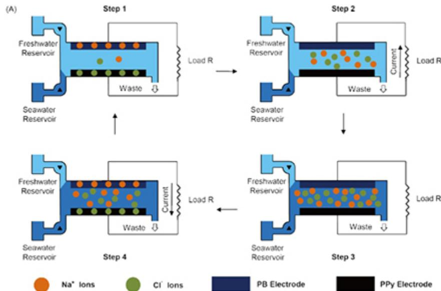
*Schematic and typical cycle representing the working mechanism of the mixing entropy battery using a Prussian Blue (PB) cationic electrode and a polypyrrole (PPy) anionic electrode.*
