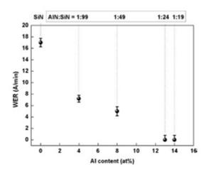
Measured wet etch rates for composite films of AIN and SiN as a function of AI content measured by XPS. The x-axis on the top of the graph indicates the AIN:SiN cycle ratio corresponding to the XPS-measured AI content displayed at the bottom. The error bars represent the standard deviation from nine measurements on the same sample.
