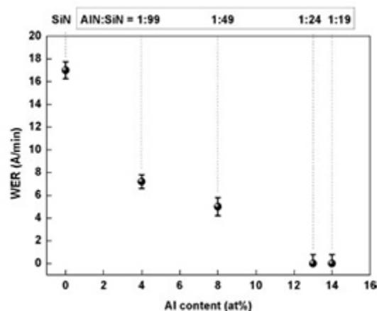
*Measured wet etch rates for composite films of AlN and SiN as a function of Al content measured by XPS. The x-axis on the top of the graph indicates the AlN:SiN cycle ratio corresponding to the XPS-measured Al content displayed at the bottom. The error bars represent the standard deviation from nine measurements on the same sample.*
