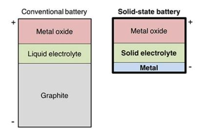
A solid electrolyte enables the use of high-performance electrode materials (e.g. lithium metal for the anode) that can dramatically improve energy density.
