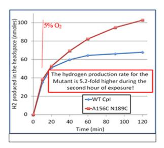
**Figure description -** Double cysteine introduction confers oxygen tolerance during hydrogen production.
