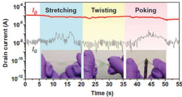
**CONPHINE TFT drain current** under stretching, twisting, and even poking by a sharp object.
