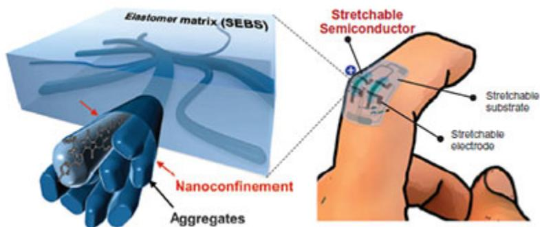
**3D morphology of the polymer semiconductor** - The increased polymer chain dynamics under nanoconfinement reduces the modulus of the conjugated polymer and delays the onset of crack formation under strain, without affecting charge mobility.
