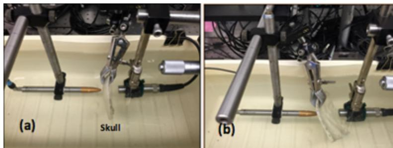
**Figure description** - Pressure field scan setup with the skull fragment placed between the transducer and hydrophone, at two different angles to emulate the normal-incident and wedge techniques (a) normal-incident transmission (b) wedge transmission.
