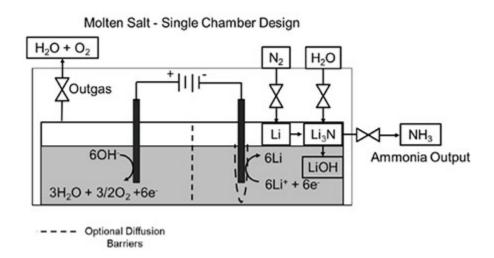
**Figure description -** A schematic of one possible set-up for an ammonia-producing system; given  $N_2$  and  $H_2O$  inputs, the system releases ammonia and byproducts  $H_2O$  and  $O_2$ .
