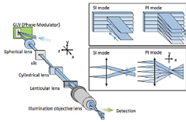
**Figure description** - Schematic of the optical setup. The light path is in the case of the SI mode.
