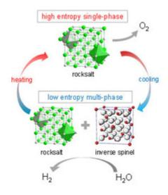
Schematic diagram of two-step thermochemical water splitting reactions using the proposed high-entropy mixed oxides.
