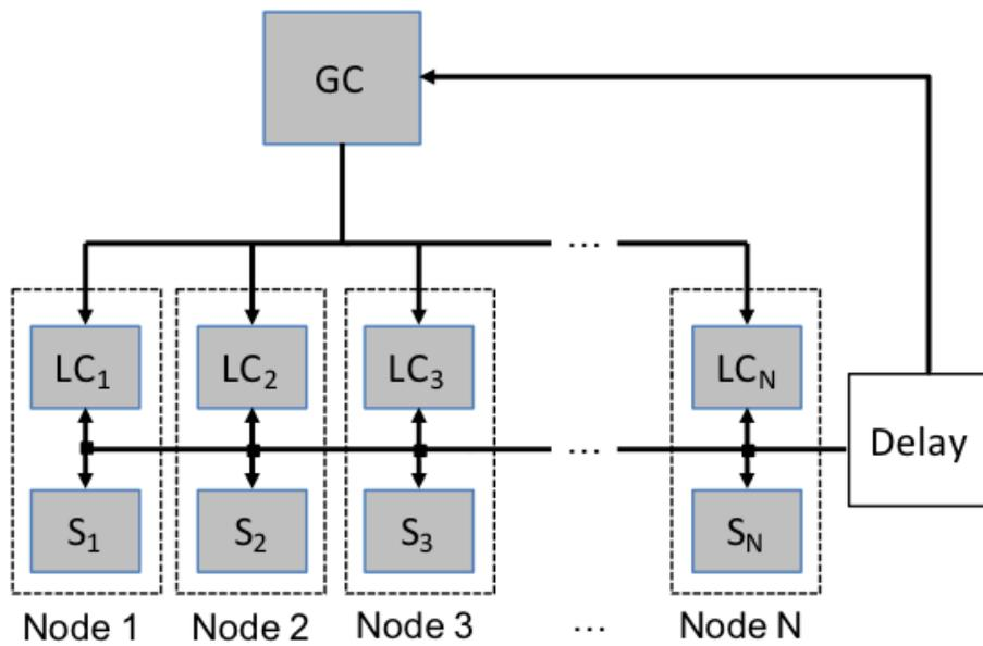
Figure 2 - Data flow in a distribution system.  $N$  customers with net loads  $S$  and local controllers LC. The local controllers communicate their data to a global controller GC, subject to a delay. The GC sends back control signals to the LCs based on the delayed information and its knowledge of the distribution network.
