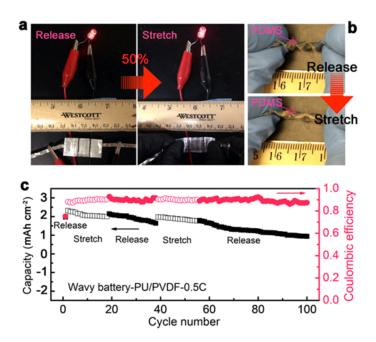
**Performances of wavy battery.** (a) light-emitting diode powered by wavy battery at released and stretchable state at 50% strain. (b) view of PDMS separator stretched to accommodate deformation. (c) Cycling performance and Coulombic efficiency for the wavy battery under releasing and stretching states (50% strain).
