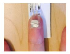
Figure description - The thin and flexible capacitive tactile sensor efficiently covers curved surfaces such as the human finger or robotic limbs
