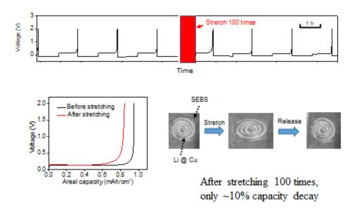
**Anode performance** when subjected to stretching during battery charging/discharging
