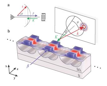
**Optomechanical antenna arrays.** A mechanical wave scatters a guided optical wave to steer a beam through a range of angles b, micron-scale antennas with guided optical and guided mechanical modes form a beam in the far-field directed into a designated angle. c, antennas are incorporated into a phased-array driven by a single piezoelectric transducer.
