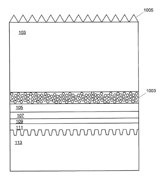
Figure 1 Example of an OLED device using a nanopatterned electrode (113), a high index internal extraction structure (IES) layer (1003) with light scattering particles to optimize outcoupling of waveguide mode, and a microlens array (1005) to optimize substrate mode.
