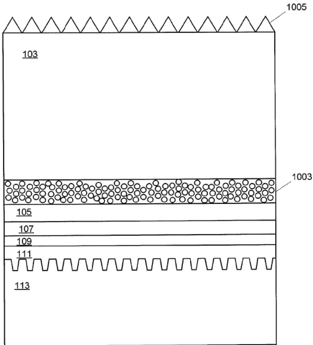
Figure 1 Example of an OLED device using a nanopatterned electrode (113), a high index internal extraction structure (IES) layer (1003) with light scattering particles to optimize outcoupling of waveguide mode, and a microlens array (1005) to optimize substrate mode.
