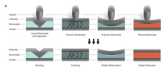
**Figure description -** a) Schematic of the response of different LIB electrolyte materials after being subjected to an impact. Liquid, ceramic, and polymer electrolytes short, crack, and deform respectively. Meanwhile, an elastic electrolyte material can reversibly recover and survive the impact event to continue operation.
