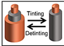
**Cross section of metal grid architecture:** Uniform opacity switching is achieved using a grid consisting of a metal core conductor (orange), surrounded by an inert metal (gray) which is covered by the electroplating outer layer metal that tints and detints the surface upon application of voltage thereby changing the opacity of the substrate.
