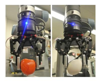
Fig. 1: An industrial robot using gecko-inspired adhesives on the gripper pads can grip and manipulate a rotten tomato and a raw egg gently and reliably.
