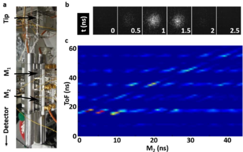
**Figure description** - Prototype of an electron cavity. An electron field emission tip and two mirrors ( $M_1$  and  $M_2$ ) are gated using high voltage RF pulsers. Both mirrors achieve sub-ns gating times (b). (c) Time resolved detected electron signal as a function of the switching time of  $M_2$ . The total intensity in each row was normalized to better visualize the signal detected after multiple round-trips, the origin was chosen arbitrarily.
