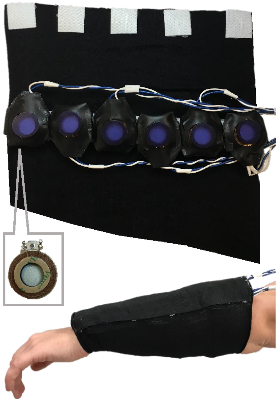
Figure 1 Device for creating the sensation of a long lateral motion
