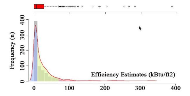
Figure 1. Efficiency Estimates of a 724 Building Subset. The red shaded region (right tail) is the 5% "most inefficient" buildings (n=38), the green shaded region is the 40% "relatively inefficient" buildings (n=292), and the blue shaded region is the 55% "relatively well performing" buildings (n=394).
