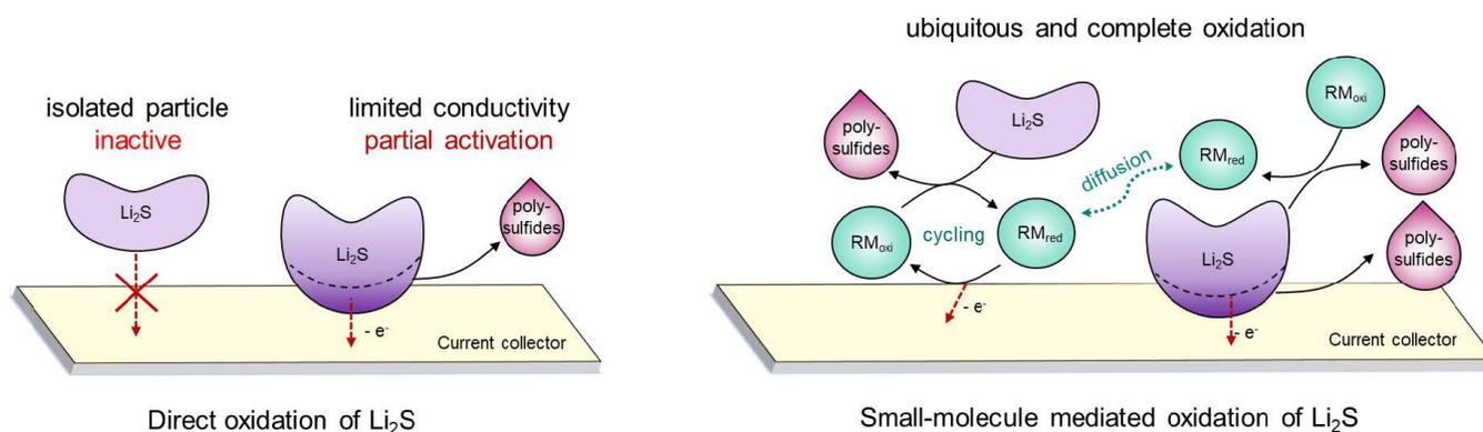
Figure 1 Direct oxidation of  $\text{Li}_2\text{S}$  vs. mediated oxidation
