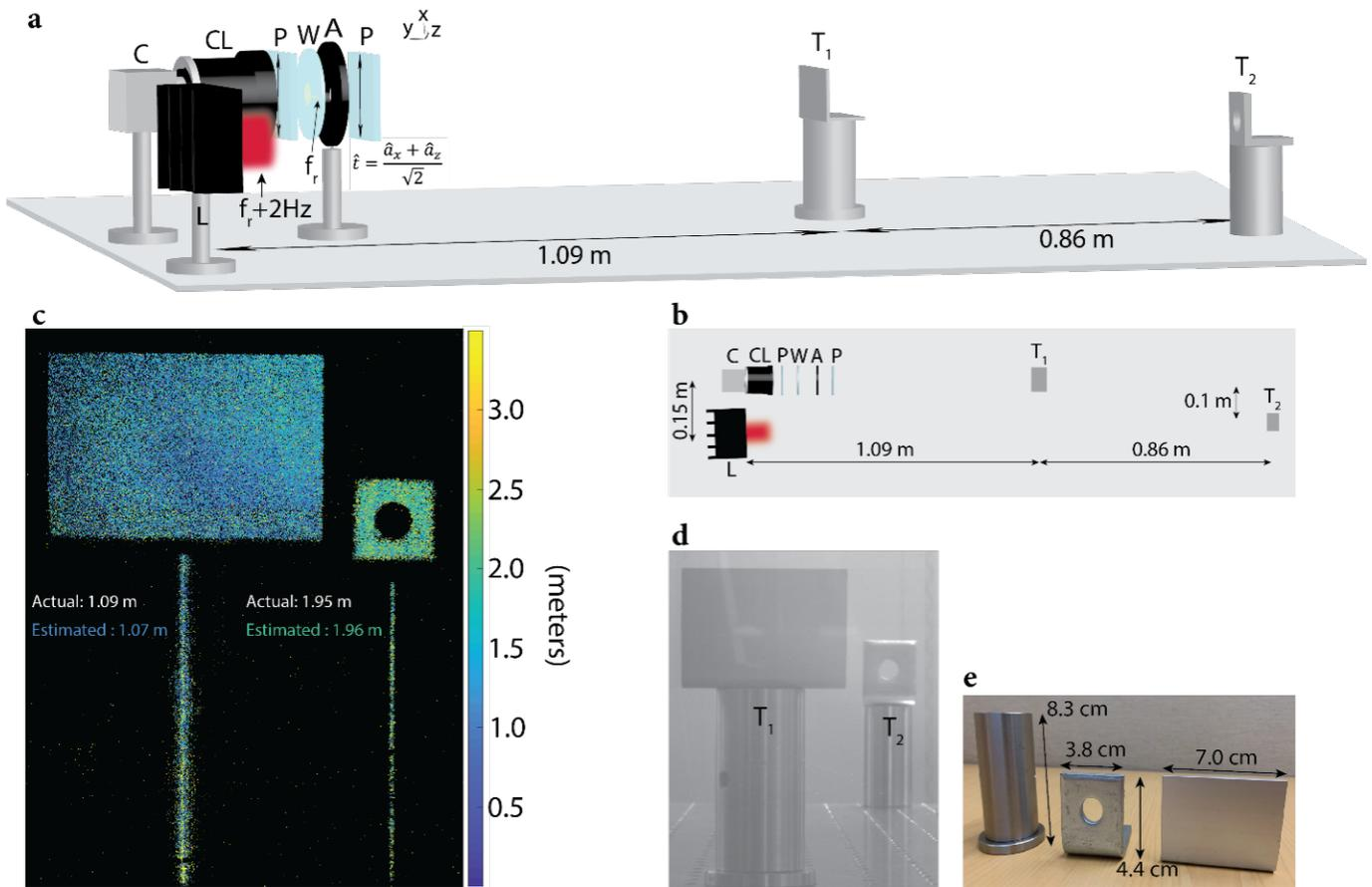
**3D imaging demonstration using the proposed system.** **a)** Schematic of the imaging system. **b)** Bird's eye view of the imaging system. **c)** Reconstructed depth map captured by the imaging system. **d)** Ambient image captured by the camera. **e)** The dimensions of the targets used for the imaging demonstration.
