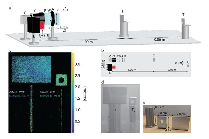
**3D imaging demonstration using the proposed system. a)** Schematic of the imaging system. **b)** Bird's eye view of the imaging system. **c)** Reconstructed depth map captured by the imaging system. **d)** Ambient image captured by the camera. **e)** The dimensions of the targets used for the imaging demonstration.
